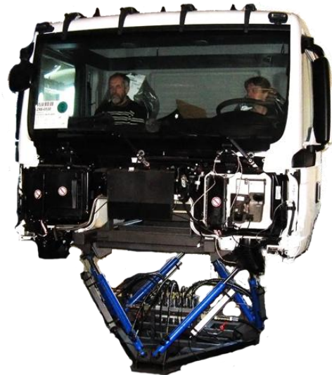
Figure 1: Truck Simulator Mounted on a Motion Platform.
