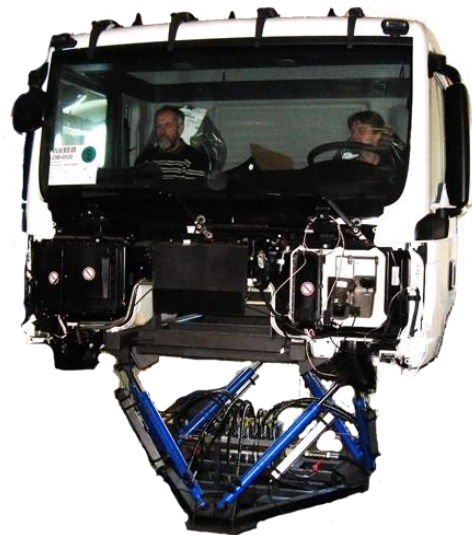
Fig. 1: Truck simulator mounted on a motion platform
